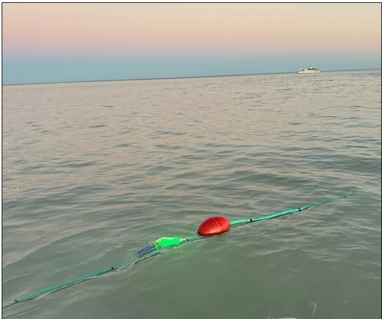
A green LED bycatch deterrent device on a gillnet deployed in Roebuck Bay, Western Australia. Photo by Dr. Alastair Harry, Western Australia Department of Primary Industries and Regional Development.
